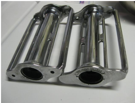
Monocoque aluminum armature – the Gibson pedal
